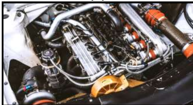
A 1985 rally Quattro's 355kW engine (evo.co.uk).
