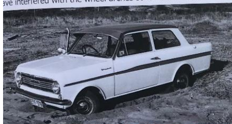
In the later cars, where the original strip was halfway down the guard/door panels, if the strip was fitted below this it would have interfered with the wheel arches so it was inverted and placed above the original strip.
