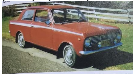
In the later cars, where the original strip was halfway down the guard/door panels, if the strip was fitted below this it would have interfered with the wheel arches so it was inverted and placed above the original strip.
