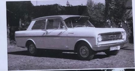
In the later cars, where the original strip was halfway down the guard/door panels, if the strip was fitted below this it would have interfered with the wheel arches so it was inverted and placed above the original strip.
