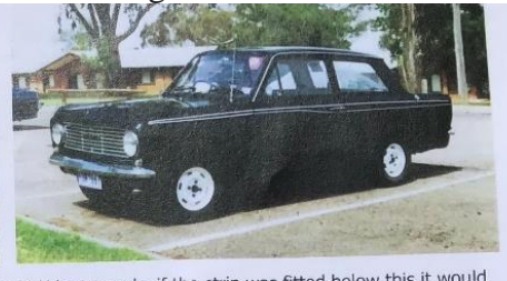
In the later cars, where the original strip was halfway down the guard/door panels, if the strip was fitted below this it would have interfered with the wheel arches so it was inverted and placed above the original strip.
