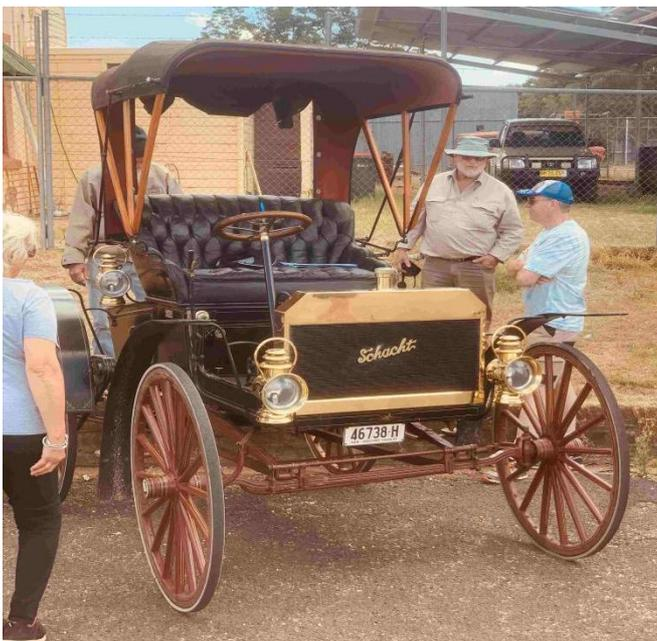
High Wheelers were mechanised horse drawn buggy's which were popular due to their high road clearance, especially in the mid-west of the USA. The popularity, cost and availability of Henry Ford's Model T and its capacity to cope with the rutted road conditions was a big part of their demise by 1915.
